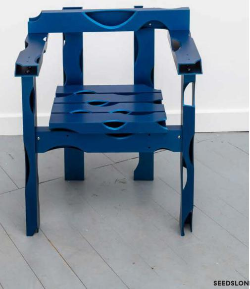
Using a standard 40 × 80 mm aluminium box section we constructed a simple armchair. The aluminium members, reminiscent of 2 × 4 timber, has sections graphically cut away revealing the hollow structure. It is a technical replica of a rustic primitive construction.
