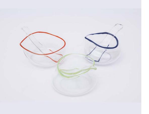
One of the processes Jochen uses is to crack glass tubes in half, this crack is often uneven as there is a chance element to the way the crack travels along the glass. He uses these irregularities to make unique shapes by melting and deforming the uneven rims, and further emphasises this by applying a coloured edge to the rim. Each bowls, spoon, carafes is unique.
